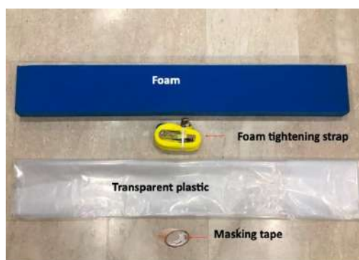
Figure 2. Material and apparatus used to assemble a gas entrapment cylinder/chamber on the RPW infested palm.
