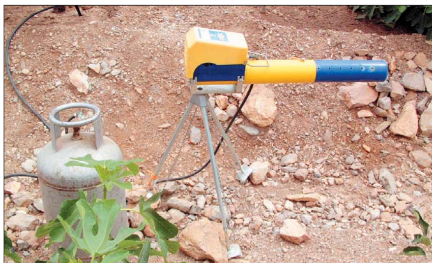
Fig. 5.4. A special gas-operated device that emits sounds to frighten the birds.
