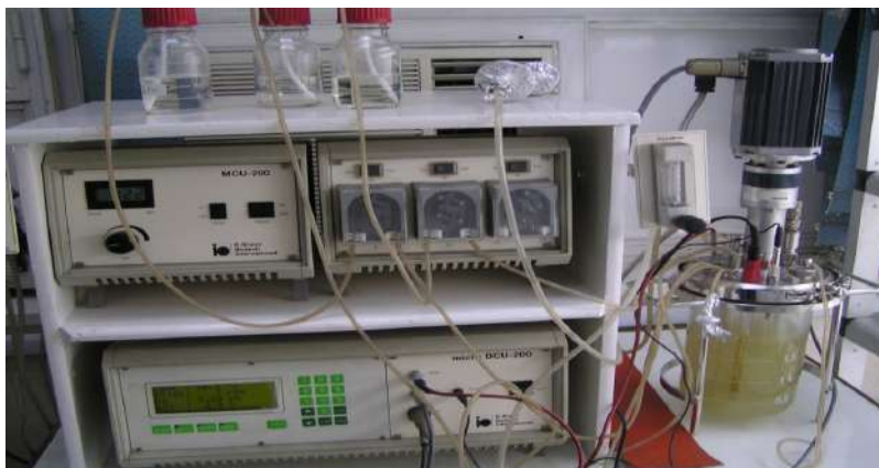
Figure 2. B-Braun Biotechnology International stirred tank bioreactor (2L).
