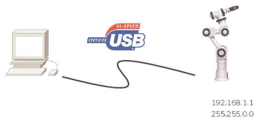
Figure 6.4: Connecting the Katana robot to a PC via USB
