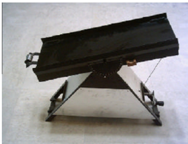
Figure 5 Apparatus for measuring static coefficient of friction (Dutta et al., 1998).
