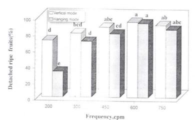
Fig. 5. Effect of frequency on detached ripe fruits at different levels of shaking mode.
