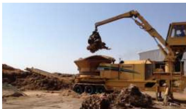
Fig. 13. Eradication of date palms severely infested by R. ferrugineus using a shredding machine (Source : J. R. Faleiro)
