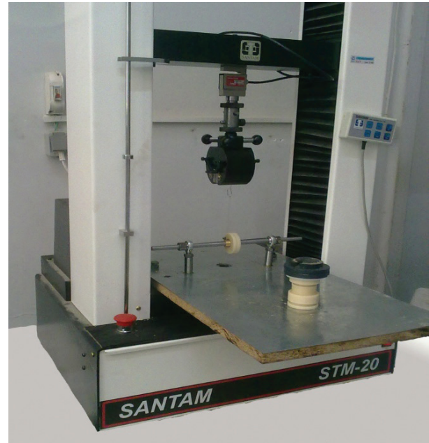
Fig. 1. Apparatus for determining the shear strength of powder
