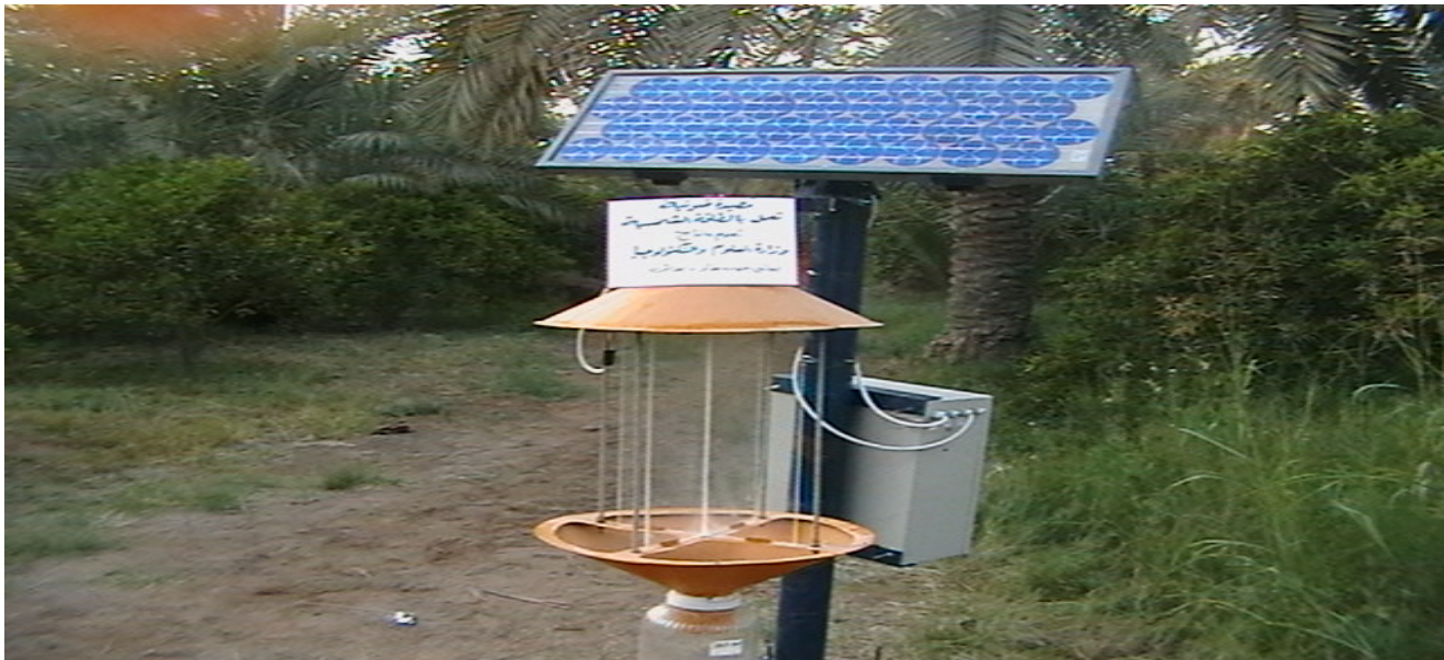
Fig.1. A locally designed solar insect light traps used to determine the population density of Oryctes elegans .
